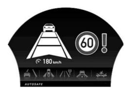
Figure 7: AUTOSAFE-Display integrated in Vehicle. The Images can be changed via Internet.
